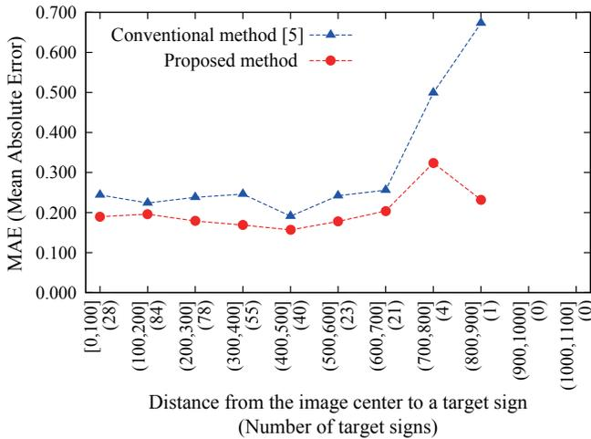
Fig. 7. Visibility estimation error according to the distance from the image center to a target.
