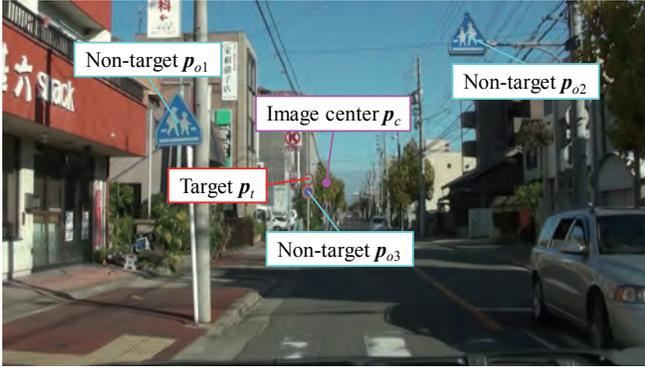
Fig. 3. Example of a target traffic sign whose centroid is  $\mathbf{p}_t$  and non-target traffic signs whose centroids are  $\mathbf{p}_{oj}$  ( $j = 1, \dots, 3$ ).
