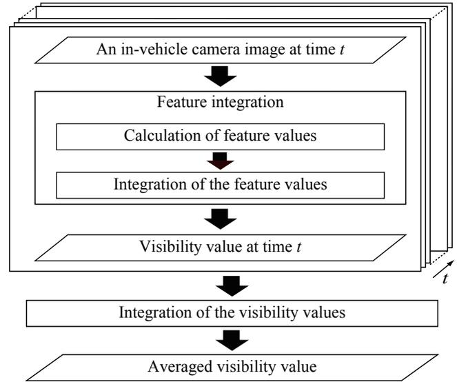
Fig. 2. Process flow of the proposed visibility estimation system.
