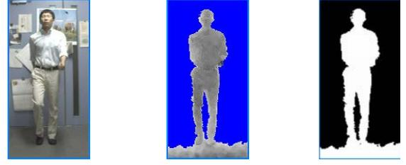
(a) Input RGB image. (b) Input depth image. (c) Segmentation result.
