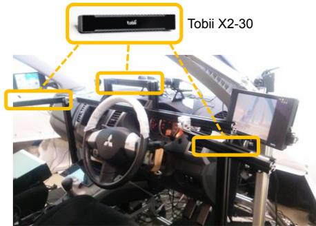
Figure 4. Three eye trackers mounted on simulator for measuring driver gaze direction
