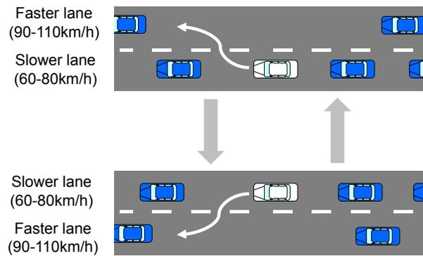
Figure 2. Traffic scenario used in the driving simulator: Drivers under time pressure make lane changes into the faster moving lane, then the faster moving lane gradually becomes congested and turns into a slower moving lane, so drivers move back into their original lane. Traffic flow alternates iteratively.
