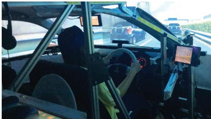
Fig. 1. Driving simulator used in the experiment.
