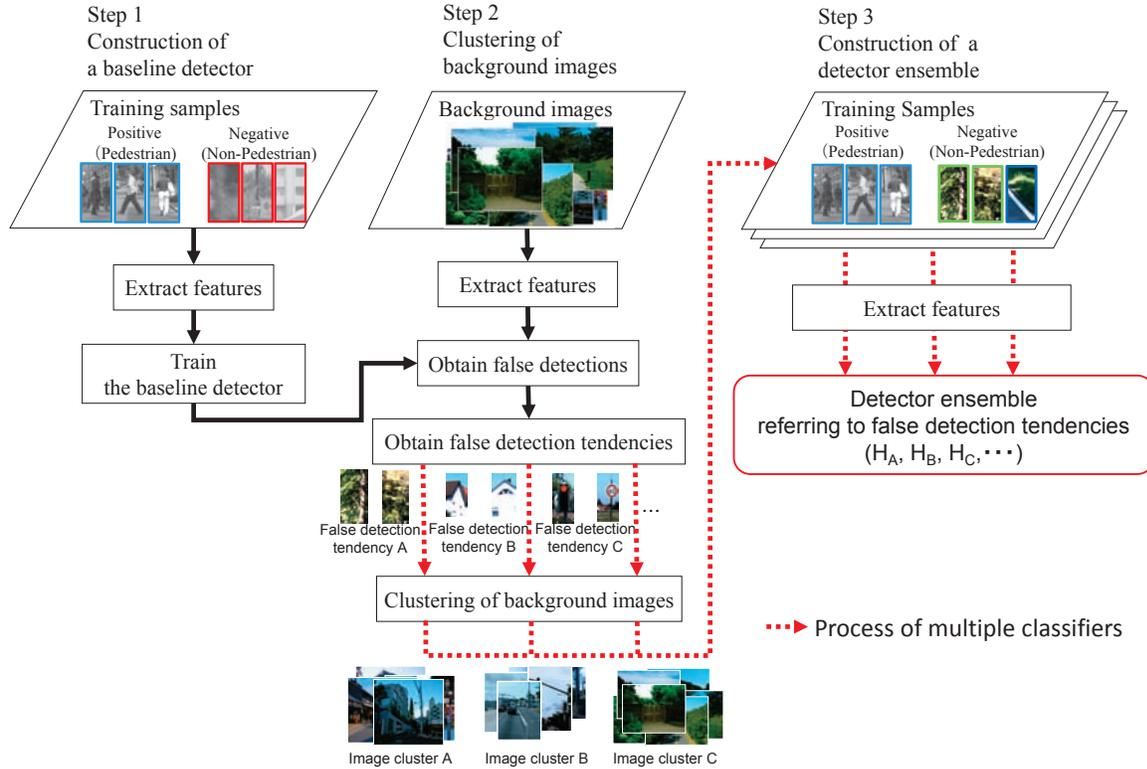
Figure 5. Training process flow of the adaptive classifier referring to false positive tendency.
