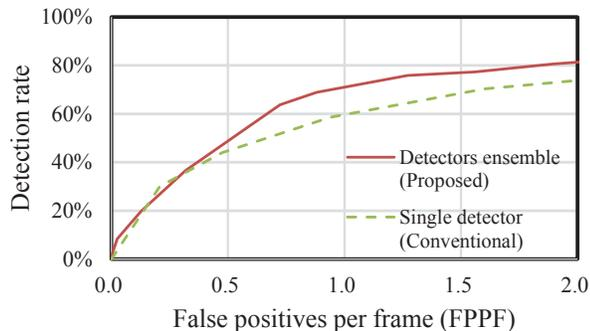
Figure 7. Detection accuracy in FROC curve.
