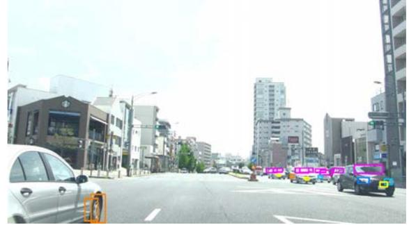
Fig. 5. Example of car parts detection result.
