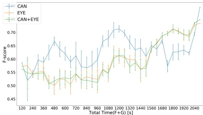
**Fig. 5:** The comparison of different feature sets. Using only the CAN data, there are some peaks at 480s, 1200s and 1680s. When we combine the driver’s blinking and driving behaviors, the trend becomes similar to the system which used only driver’s blinking.
