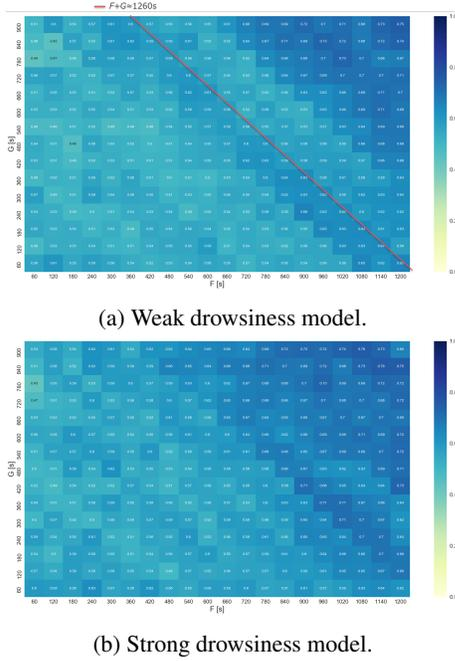
**Fig. 2:** F-score of drowsiness sign detection model. The x-axis denotes the length of  $F$ , and the y-axis denotes the length of  $G$ . The F-scores are in the range of  $0-1$  and are presented with yellow-green-blue colors. In the weak model, the red line presents the area where  $F+G$  is about 1260s.
