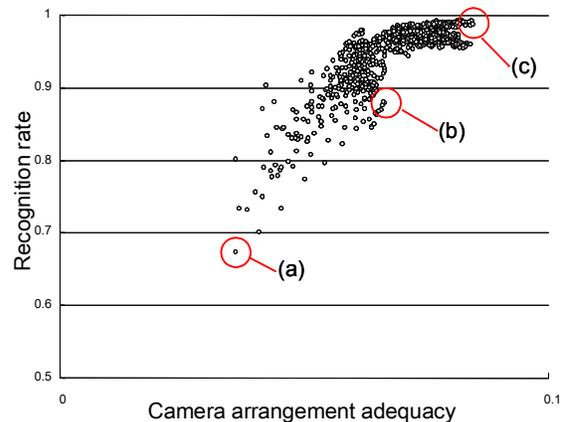
Figure 6: Relation between FP recognition rates in middle resolution case and camera arrangement adequacies: arrangements (a), (b), and (c) correspond to arrangements in Table 1
