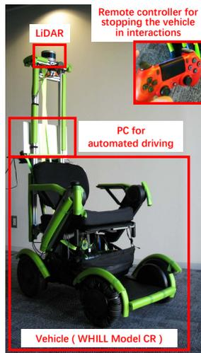
Fig. 3: Experimental vehicle.
