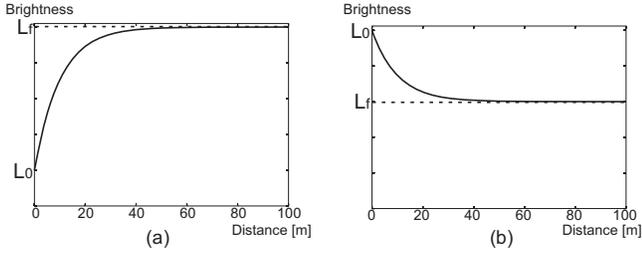
Fig. 2. The brightness degradation with distance ( $k = 0.1$ ): (a)  $L_0$  is smaller than  $L_f$ ; (b)  $L_0$  is bigger than  $L_f$ .
