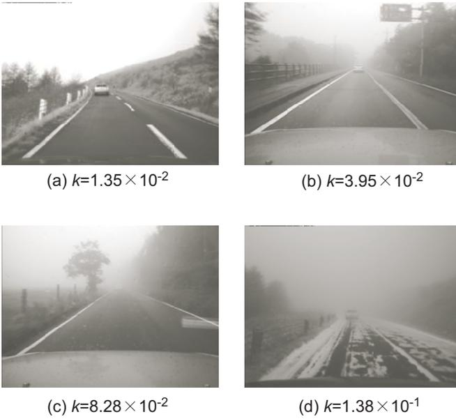
Fig. 8. Extinction coefficients for various weather conditions
