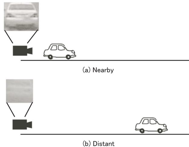
Fig. 1. The visibility of a preceding vehicle depends on distance.
