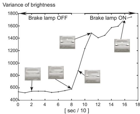
Fig. 10. Change of variance of brightness by lighting of brake lamps
