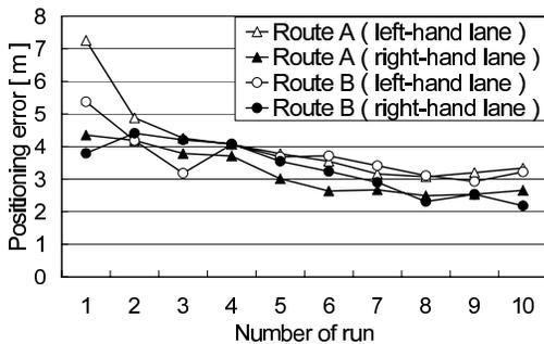
Fig. 10. Relation between number of runs and positioning error of averaged navigation GPS coordinates.
