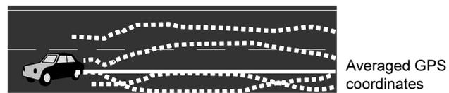
Fig. 5. Improving position information of Range Data Map by averaging vehicle locations. Continuous line represents averaged positions. Broken lines represent positions obtained by GPS.
