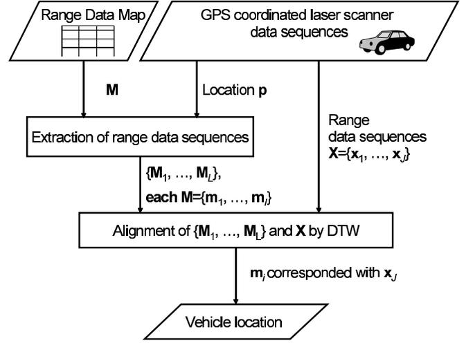
Fig. 7. Flow chart of vehicle localization scheme.
