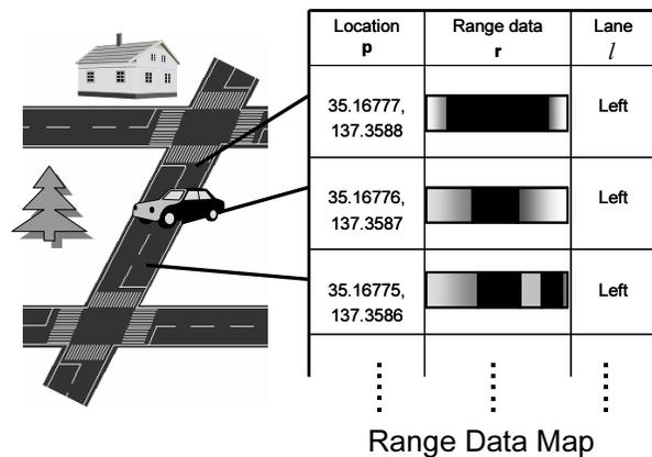
Fig. 4. Part of Range Data Map.  $\mathbf{p}$  represents location vector with latitude and longitude.  $\mathbf{r}$  represents range image at location, where intensity is inversely proportional to depth.  $l$  represents lane.
