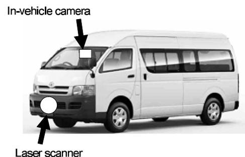
Fig. 1. Position of laser scanner and in-vehicle camera mounted on vehicle used in experiments.
