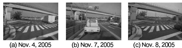
Fig. 8. Examples of in-vehicle camera images synchronized with aligned range data measured on different days. The date is indicated under each image. In this case, we aligned (a) with the other three. The alignments succeeded in (c). They failed in (b), because of a vehicle in front waiting for a traffic signal to change.
