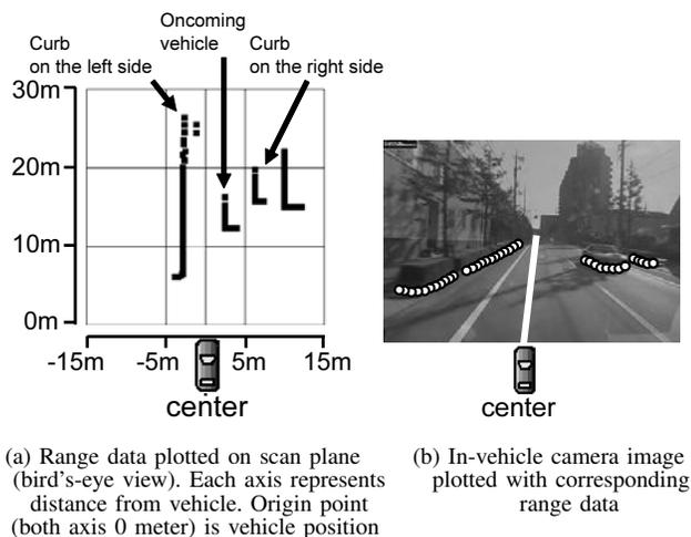
Fig. 2. Range data and in-vehicle camera image at same location: curbs and an oncoming vehicle are observed. Since the mounted positions of the devices are different, the plotted range data in (b) do not form horizontal lines.
