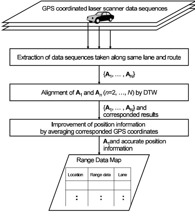
Fig. 6. Flow chart of construction of Range Data Map.
