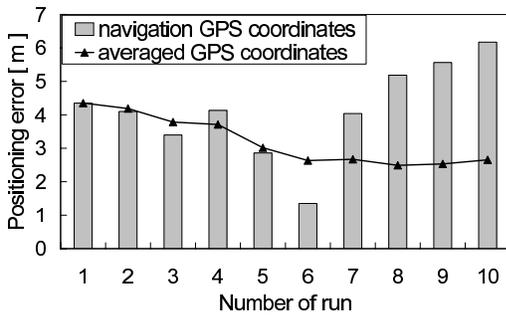
Fig. 9. Positioning error of averaged GPS coordinates by number of runs and of navigation GPS coordinates for each run.
