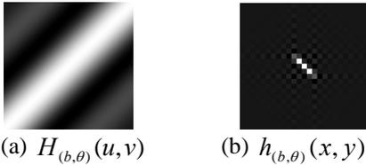
Fig. 2. Example of motion-blur PSF ( $b = 5, \theta = \pi/4$ ).
