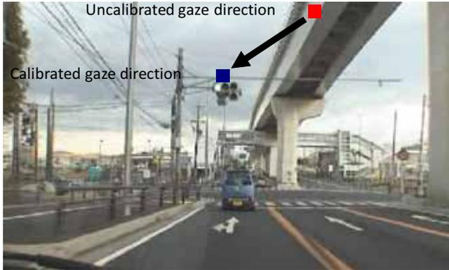
Fig. 8. Example of calibrated result when driver gazed at a traffic signal.
