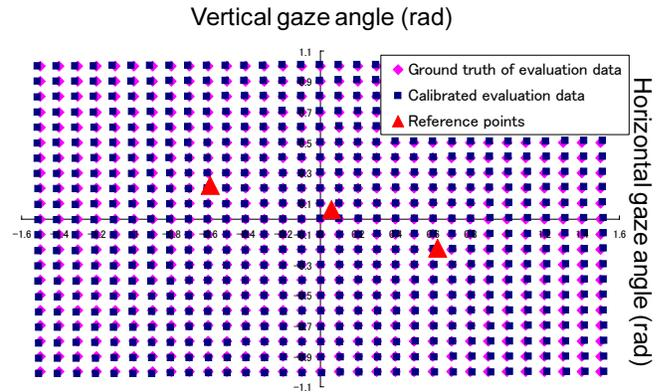
Fig. 7. Results of calibration using three reference points.
