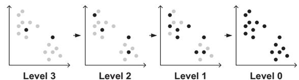
Fig. 1. Illustration of the technique of hierarchical data sampling. The black dots represent the data (vectors) that are used for K-Means in each hierarchical level.
